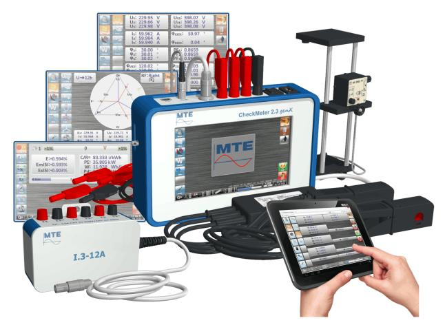
The CheckMeter 2.3 genX Portable Standard Meter is a threephase portable electronic meter test unit of accuracy class 0.2, used for testing single- and three-phase electricity meters on-site.
